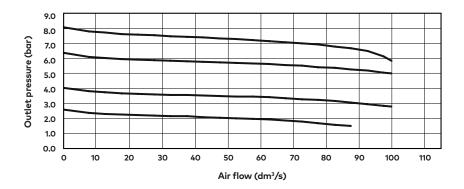
Inlet pressure: 10 bar (145 psi) Port size: 3/8", 40 µm element
