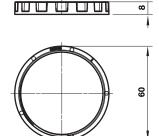
Recommended panel hole size: ø 55 mm ... 57 mm Panel thickness: 2 ... 6 mm
