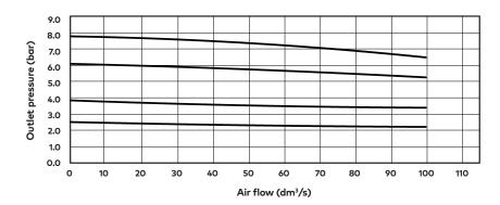
Inlet pressure: 10 bar (145 psi) Port size: 3/8", 5 µm element
