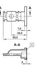
1 'O'-ring (included in scope of supply of bracket)
